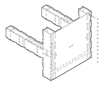
Note the 'zip' seams where two panels meet, transferring forces along the skin of the structure.
