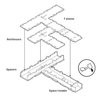
The full box-frames are assembled from four types of part.
