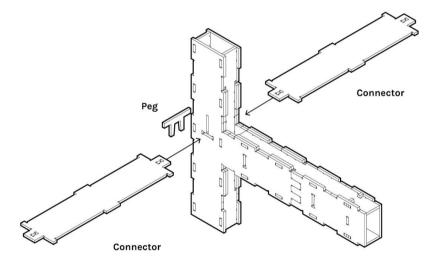
Connectors are generic; generally there are only two types. 'Primary' connectors slot in during the barn-raising, and are pegged into place. 'secondary' connectors just slot into place after the frames have been raised. Generally you only need connectors at the corners, but you will also need to put them in to support floor panels etc.
