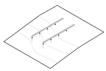
The WikiHouse chassis system can be used on more or less any site, including sloping sites, however the site must provide 2 or more 'rails' (usually timber joists) which are parallel and level. These 'rails' can be supported by almost any kind of foundation type (eg screw piles, concrete trench foundations, adjustable pads etc.) They can also 'step' down a hill if required. The chassis can then be assembled onto those rails, and bolted to them using steel brackets.
