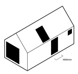
This leaves a clear opening size of 1050mm for windows and doors along the side walls, roof and floor. Within these rules, openings can be positioned more or less anywhere in the design.
