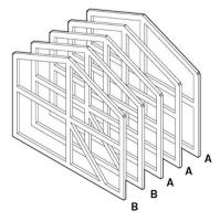
Each complete box frame has a letter, eg a house might have several type 'A' frames, a few type 'B' frames etc. The order of these can be understood like a DNA chain along the house. eg. A, A, B, B, A. So the first F piece in frame type A would be called '**A/F1'** for example.
