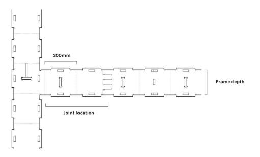
The frame profile has a set 'depth'. The default frame depth is 250mm, though it can be lower (min 200mm) for smaller structures or higher for larger ones. Download the sketchup model and turn on 'hidden geometry' and 'colour by layer'. You will see that the frame is quite easy to build in sketchup, since it mostly comprises of a repetitive grammar of 300mm long lego-like modules.
